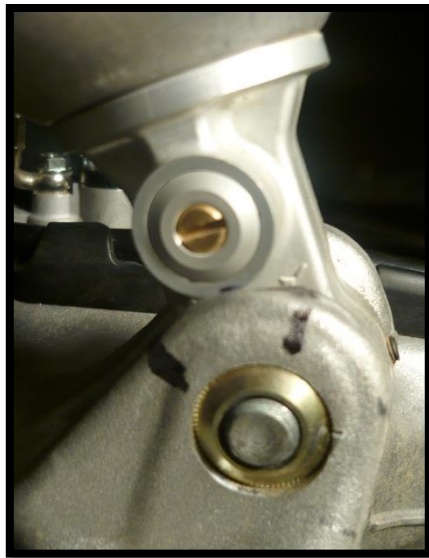
REMOVE SPRING. ROTATE SWINGARM. MARK SHOCK FOR MOVEMENT LOCATION
